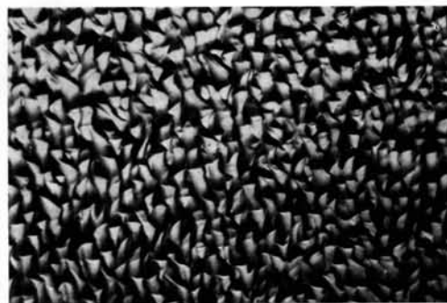
Fig. 13. Cleavage surface deeply etched with water vapor. 330 × .
