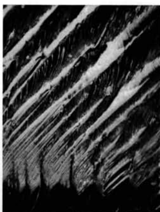
Fig. 2. Fractograph of ADP crystal in preceding figure, taken with dark-field illumination. 40 \times .
