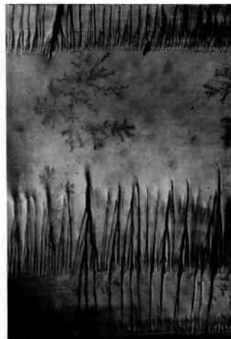
Fig. 9. Fractograph revealing an elaborate dendritic structure on the cleavage facet. 56 × .
