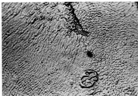
Fig. 12. Cleavage facet lightly etched with water vapor. 180 × .
