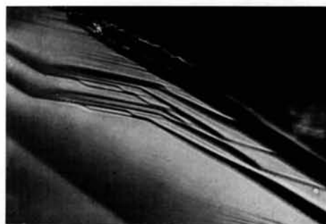
Fig. 6. Hackle surface at higher magnification, showing an indication of crystallographic and lamellar effects. 310 \times .
