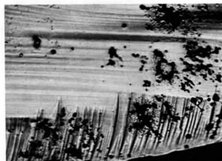
Fig. 11. Deep pitlike markings on a hackle surface, possibly representing cross-sections of the dendrite-type defects shown in the two preceding figures. 180 × .
