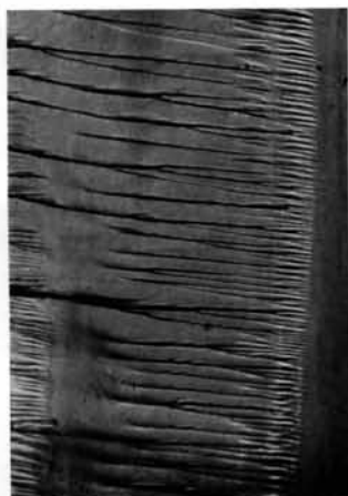
Fig. 4. Fractograph showing typical hackle structure. 96 \times .
